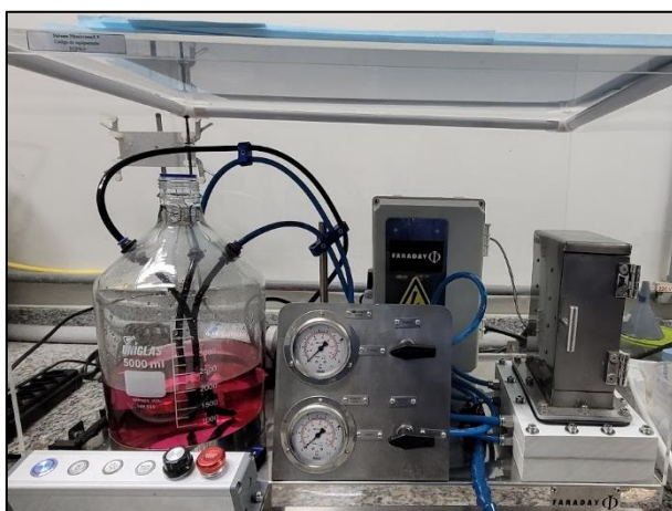
Figure 1: Cross-flow permeation system with recirculation of permeate and retentate.
